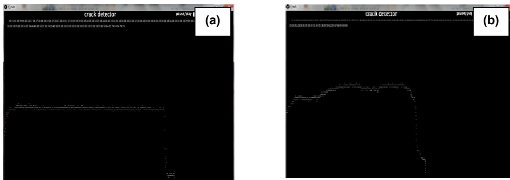
Fig. 5. Result from the tested done galvanized pipe (a) without defects (b) with longitudinal defects in section 1
