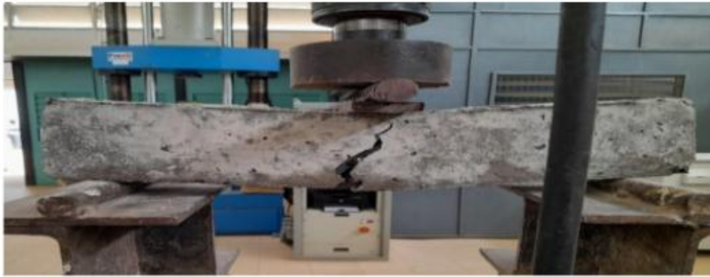
Fig. 9. Ductile failure of specimen with high volume of tire aggregate after flexural test
