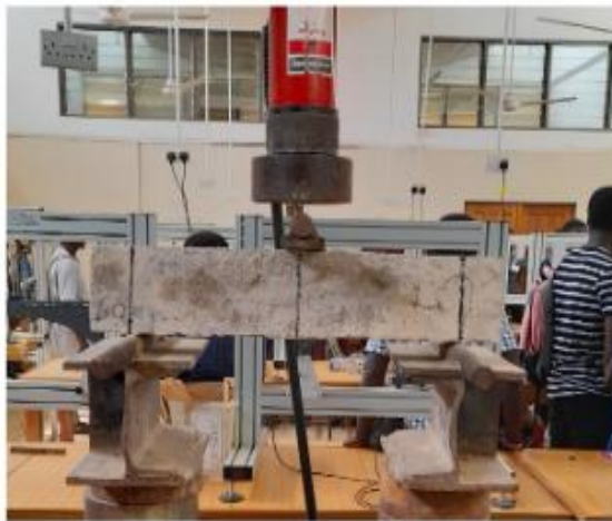
Fig. 2. Modulus of rupture test
