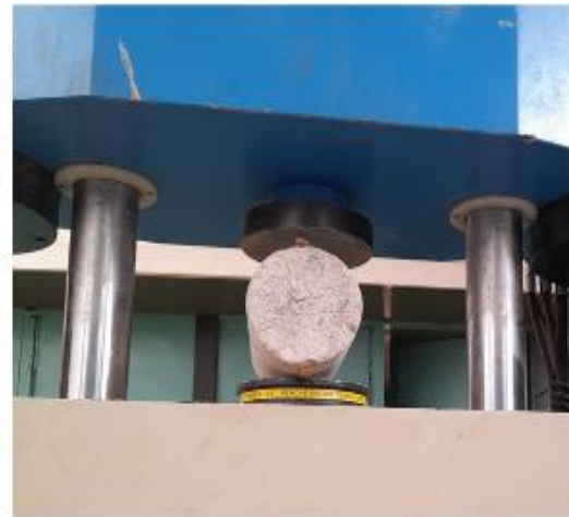
Fig. 3. Split tensile test
