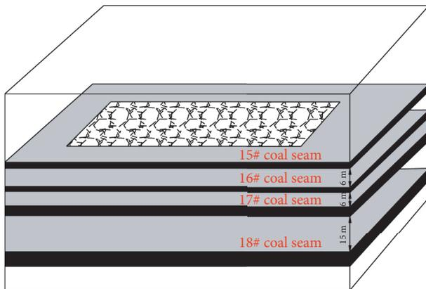
FIGURE 2: Schematic diagram of the spatial position relationship of coal seams.
