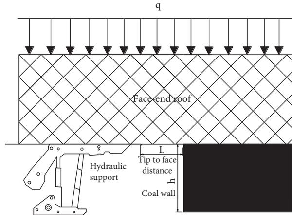
FIGURE 4: “Face-end roof-coal wall-support” model.
