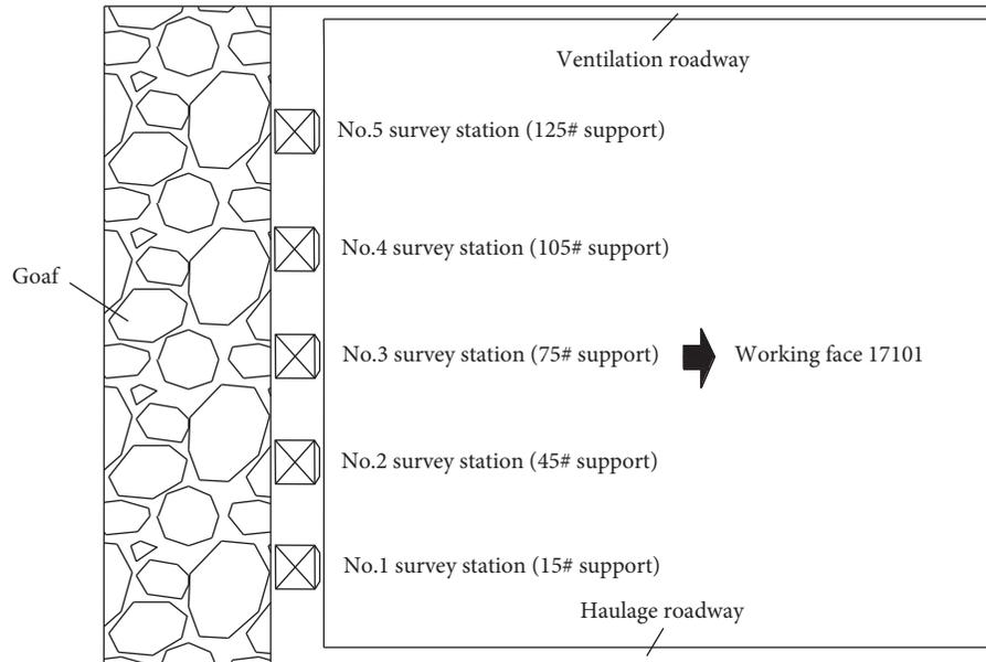
FIGURE 3: Layout of mine pressure observation stations at working face 17101 under repeated mining.
