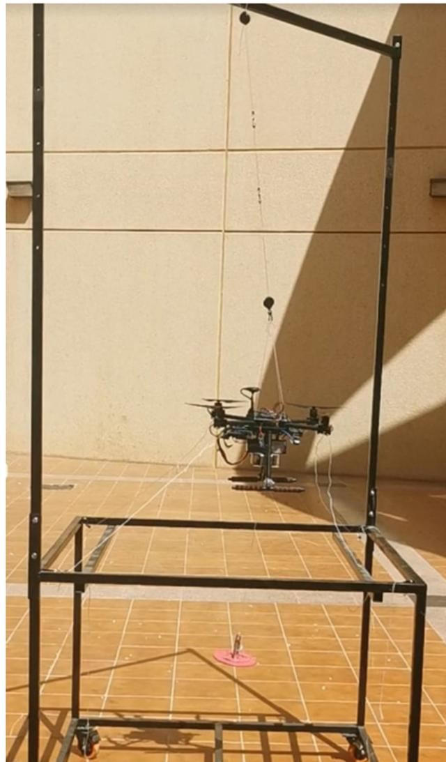
**Figure 12.** Restricted quadrotor with a suspended load in the test platform.
