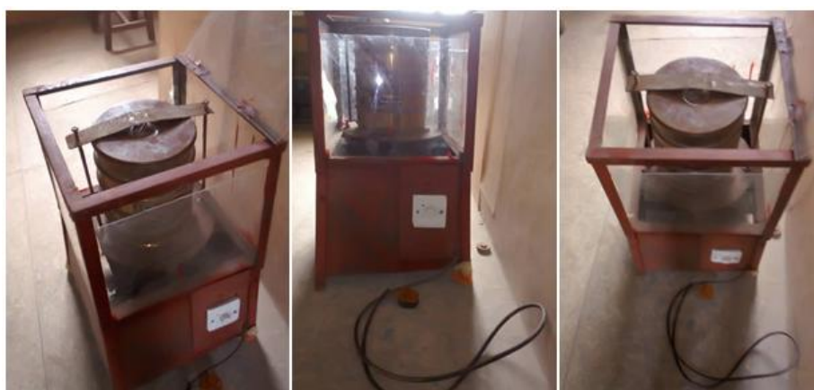
Fig. 3. Schematic of the fabricated mechanical sieve shaker
