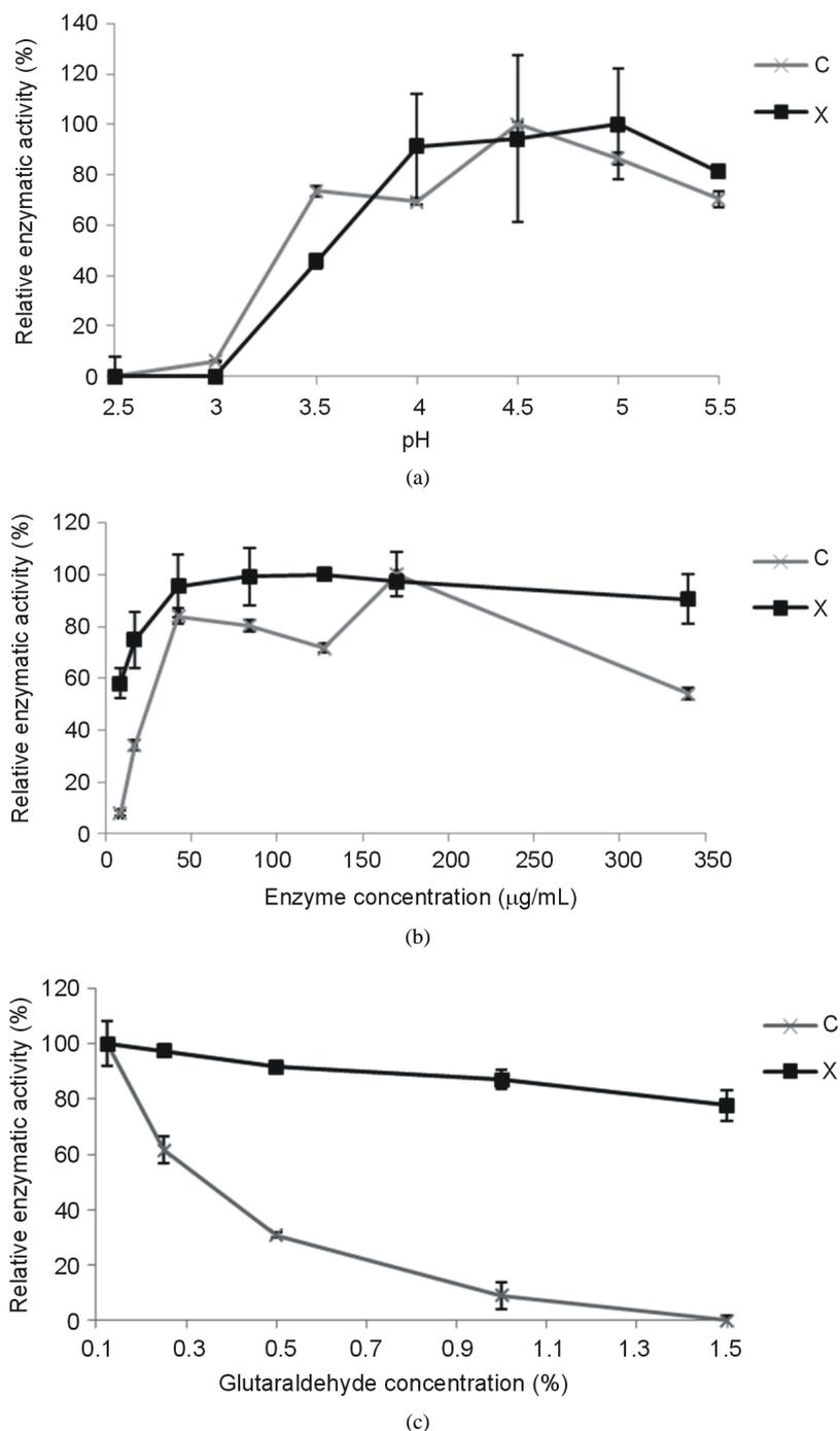
**Figure 1.** Effect of different conditions on the activity of immobilized cellulase (C) and xylanase (X). (a) Optimal pH; (b) Optimal enzyme concentration; (c) Optimal glutaraldehyde concentration. Relative activity was calculated by taking maximum enzyme activity as 100% in each case.
