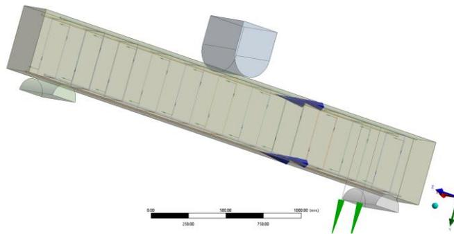
Fig. 1. Reinforced concrete beam model
